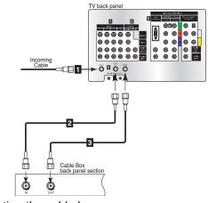
Figure 3. Connecting the cable box.
